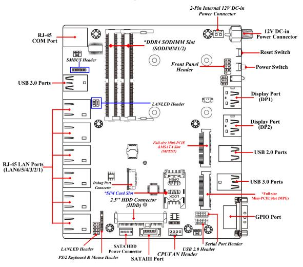
Note: SIM card slot only work when compatible SIM card installed & 3G LAN card installed in MPE Mini-PCIE slot.
