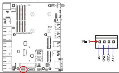
**Warning:** Make sure that Pin-1 of compatible SATA Power connector is inserted into corresponding Pin-1 of SATAPW to avoid possible damage to the board and hard disk driver!
