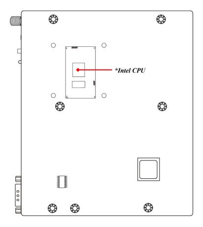
\*Note: CPU is the most important part of the board and very fragile to any possible harm. Make sure that there is no damage to the CPU during any installation procedures!
