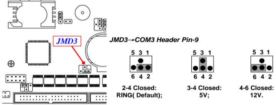
\*Note: JMD3 is only optional for NF695HV series models with COM3 serial port header(from COM3-6 combo block).
