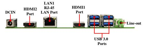
**Warning!!**The board has a 12V DC-in power connector (**DCIN3**) in I/O back panel and an internal 12V power connector (DCIN2). User can only connect one type of compatible power supply to one of them to power the system.
