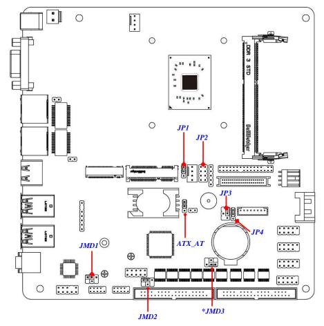
\*Note: the diagram above is from NF695HV series and serves as illustration purpose only. JMD3 is optional to NF695HV series models, please refer to the model you purchased for actual specifications.
