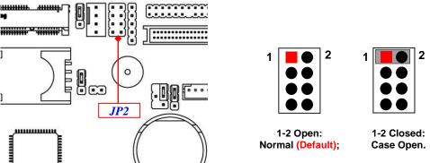
**Pin (1-2) Close:** When Case Open function pin short to GND, the Case Open function was detected. When Used, needs to enter BIOS and enable 'Case Open Detect' function. In this case if your case is removed, next time when you restart your computer, a message will be displayed on screen to inform you of this.
