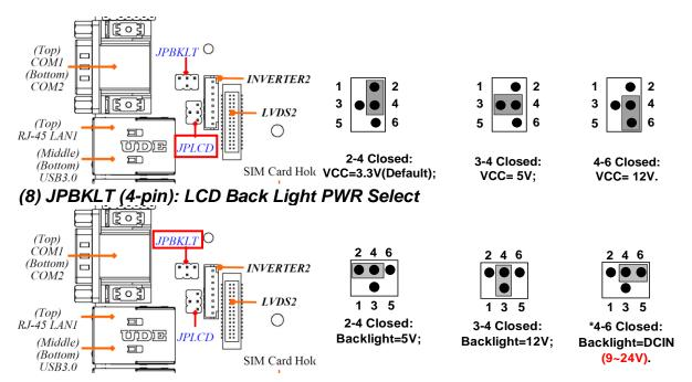
\*Note: In the case that JPBKLT is set as Pin(4-6) closed, backlight power VCC is the same as adapter voltage value (wide voltage range from 9V to 24V).
