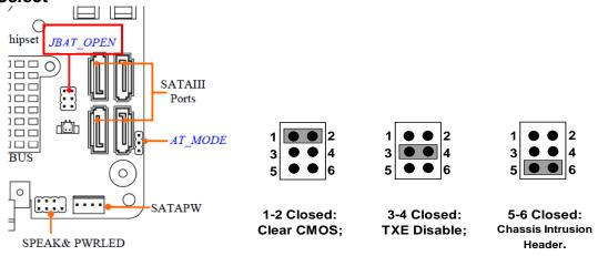
(2) AT\_MODE (3-pin): AT/ATX Mode Select
