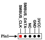
(9) PS2KBMS (6-pin): PS2 Keyboard & Mouse Port Header Pitch=2.54mm
