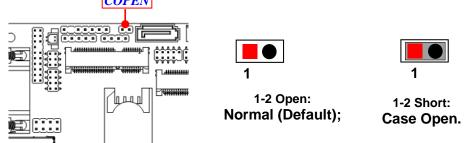
**Pin (1-2) Close:** When Case Open function pin short to GND, the Case Open function was detected. When Used, needs to enter BIOS and enable 'Case Open Detect' function. In this case if your case is removed, next time when you restart your computer, a message will be displayed on screen to inform you of this.
