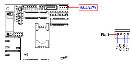
*Warning:* Make sure that Pin-1 of compatible SATA Power connector is inserted into corresponding Pin-1 of SATAPW to avoid possible damage to the board and hard disk driver!
