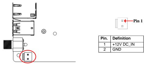
**Warning!!** The board has a 12V DC-in power connector (DC\_IN) in I/O back panel and an internal ATX2P (ATXPWR) power connector. User can only connect one type of compatible power supply to one of them to power the system.
