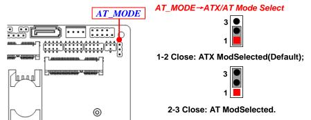
\*ATX Mode Selected: Press power button to power on after power input ready; AT Mode Selected: Directly power on as power input ready. COPEN (2-pin): Case Open Message Display Function Select Pitch=2.54mm
