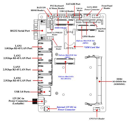
Note: SIM card slot only work when compatible SIM card installed & 3G LAN card installed in MPE1 Mini-PCIE slot.
