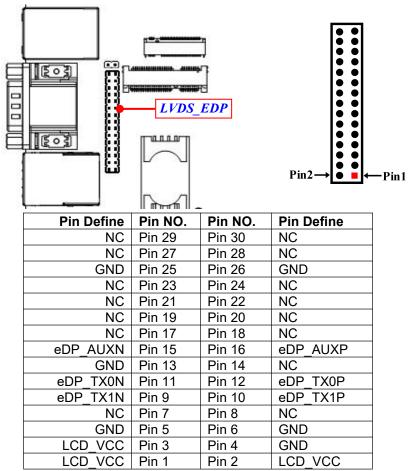
\*Note: LVDS\_EDP functions as LVDS and EDP Combo header. User aslo needs to go to BIOS to set 'LCD Panel Type' (refer to Page-43) to before connecting compatible cable to the header.
