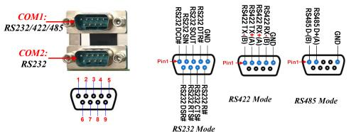
COM1 port can function as RS232/422/485 port. In normal settings COM1 functions as RS232 port. With compatible COM cable COM1 can function as RS422 or RS 485 port. User also needs to go to BIOS to set '**Transmission Mode Select**' for COM1 at first, before using specialized cable to connect different pins of this port.
