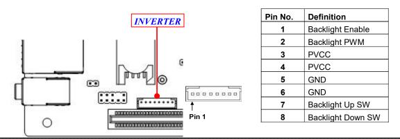
**Warning!** Find **Pin-1** location of the inverter and make sure that the installation direction is correct! Otherwise serious harm will occur to the board/display panel!!
