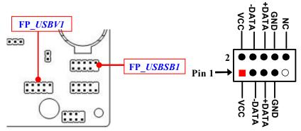
(7) FP\_USBSB1 (9-pin): USB 2.0 Port Header POWER: STANDBY POWER (5VSB) with wake up function
