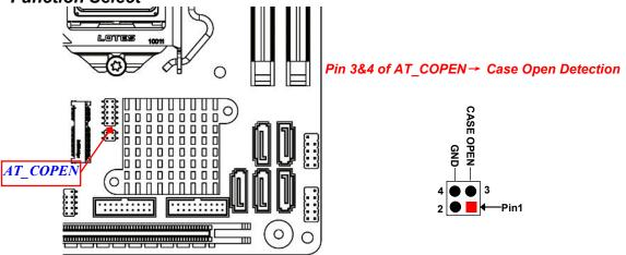
**Pin (3&4) Closed**: When Case open function pin short to GND, the Case open function was detected. When used, needs to enter BIOS and enable 'Case Open Detect' function. In this case if your case is removed, next time when you restart your computer, a message will be displayed on screen to inform you of this.
