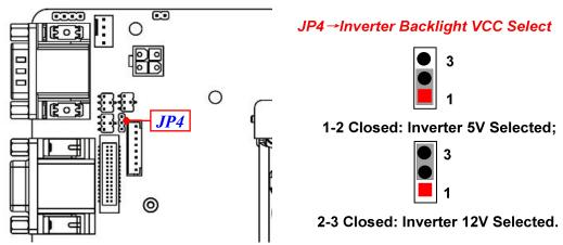
\*Note: Maximum current limit is 1.5A while using 5V or 12V.
