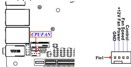
\*Note: Maximum current limit is 1.5A while using 12V working voltage.
