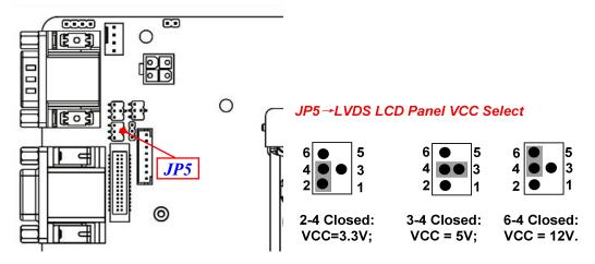
\*Note: Maximum current limit is 3A while using 3.3V, 5V or 12V.
