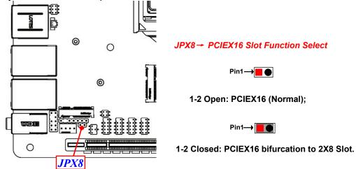
\*Pin (1-2) Open: Normal function as PCIEx16 slot;
