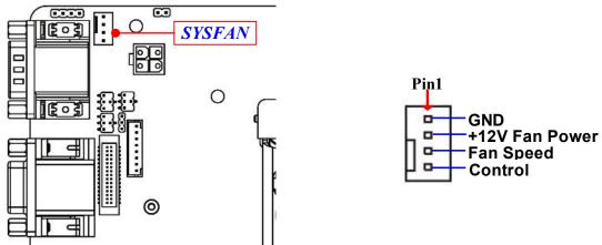
\*Note: Maximum current limit is 1.5A while using 12V working voltage.
