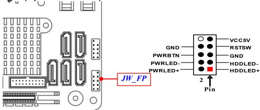
\*Note: Maximum current limit is 1A while using 5V working voltage.
