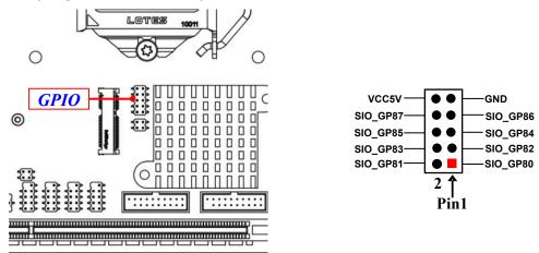
\*Note: Maximum current limit is 1A while using 5V working voltage.
