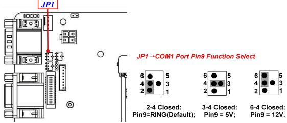
\*Note:Maximum current limit is 500mA while using 5V or 12V.
