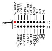
\*Note: Maximum current limit is 1.5A in total while using 5V working voltage.
