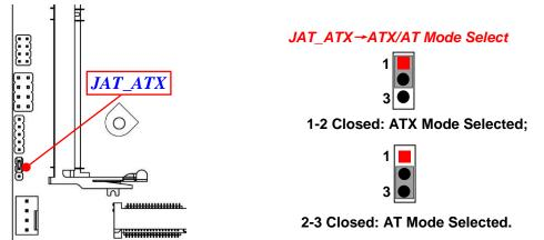
\*ATX Mode Selected: Press power button to power on after power input ready; AT Mode Selected: Directly power on as power input ready.
