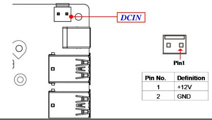
Warning: Find Pin-1 position before connecting power cable to this 2-pin power connector. WRONG INSTALLATION DIRECTION WILL DAMAGE THE BOARD!!
