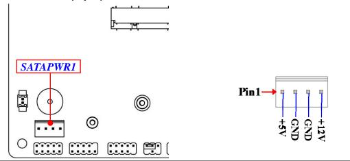
*Warning:* Make sure that Pin-1 of compatible SATA Power connector is inserted into corresponding Pin-1 of **SATAPWR1** connector to avoid possible damage to the board and hard disk driver!
