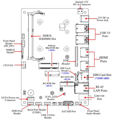
\*Note: 1. SIM card slot (SIMCARD/JSIM header expansion card) only work when compatible SIM card installed & LAN expansion card installed in the full-size MPE slot (MPE); 2. SIMCARD and JSIM is optional, i.e., only one can work at the same time.
