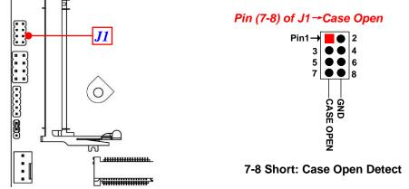
**Pin 7-8 Short**: When Case open function pin short to GND, the Case open function was detected. When Used, needs to enter BIOS and enable '**Case Open Detect**' function. In this case if your case is removed, next time when you restart your computer, a message will be displayed on screen to inform you of this.
