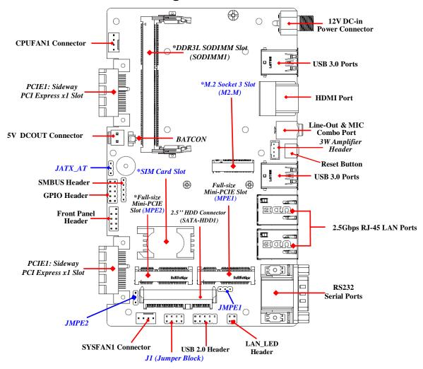
Note: 1. The memory module should be DDR3L 1.35V SODIMM and not exceeding 8GB total capacity. 2. SIM card slot only work when compatible SIM card installed & 3G LAN card installed in MPE2 Mini-PCIE slot.
