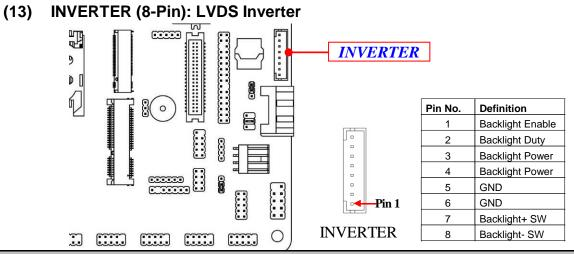
*Warning!* Find Pin-1 location of the inverter and make sure that the installation direction is correct! Otherwise serious harm will occur to the board/display panel!!
