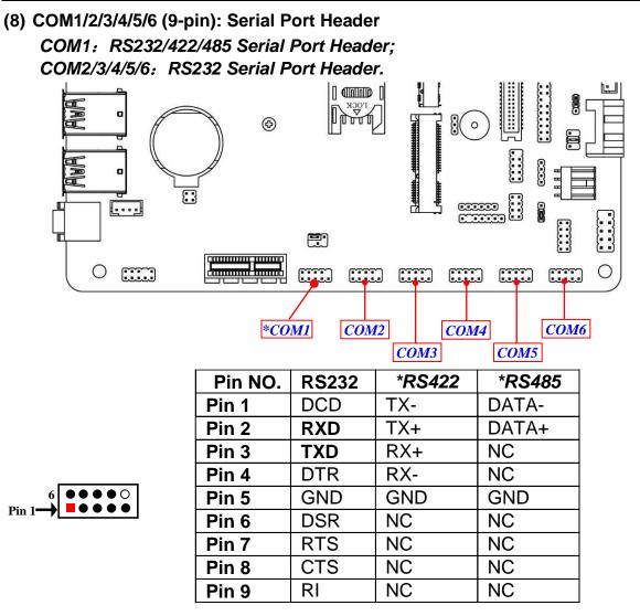
\*Note: In the case that COM1 header supports RS422, RS485 function, besides connecting compatible COM cable for RS422 or RS 485 function, user also needs to go to BIOS to set corresponding '**Transmission Mode Select'** for COM1 (refer to Page-28).
