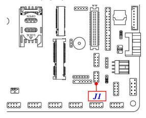
Pin 3&4 of J1(8-pin): RTC Reset
