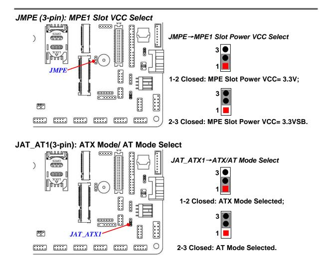
**ATX Mode Selected**: Press power button to power on after power input ready; **AT Mode Selected**: Directly power on as power input ready.
