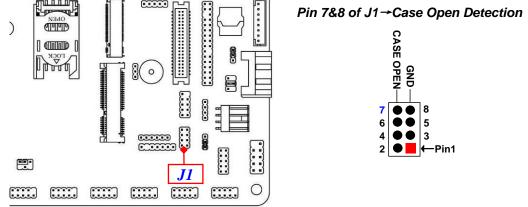
**Pin (7&8) Closed**: When Case open function pin short to GND, the Case open function was detected. When used, needs to enter BIOS and enable 'Case Open Detect' function. In this case if your case is removed, next time when you restart your computer, a message will be displayed on screen to inform you of this.
