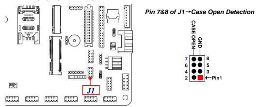
**Pin (7&8) Closed**: When Case open function pin short to GND, the Case open function was detected. When used, needs to enter BIOS and enable 'Case Open Detect' function. In this case if your case is removed, next time when you restart your computer, a message will be displayed on screen to inform you of this.
