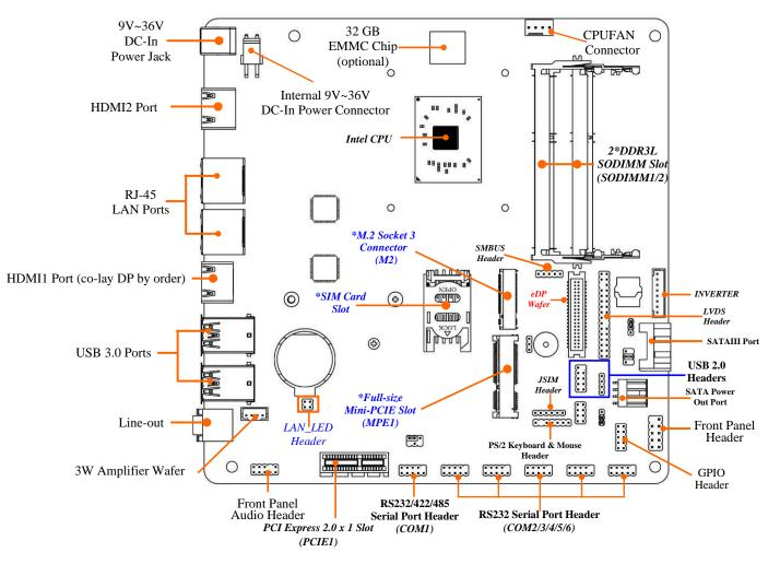
\*Note: 1. SIM card slot (SIMCARD/ expansion card drawn from JSIM header) only work when compatible SIM card installed & LAN expansion card installed in the full-size MPE slot (MPE1); 2. SIMCARD and JSIM is optional, i.e., only one can work at the same time.
