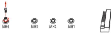
2. Remove the screw post and nut fixed at location **MH4** by default (Skip step 2 & 3 and go straight to Step 4 if you are going to use the default nut).
