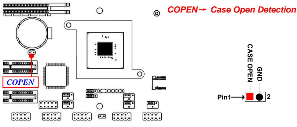
**Pin 1-2 Short:** When Case open function pin short to GND, the Case open function was detected. When Used, needs to enter BIOS and enable 'Case Open Detect' function. In this case if your case is removed, next time when you restart your computer, a message will be displayed on screen to inform you of this.
