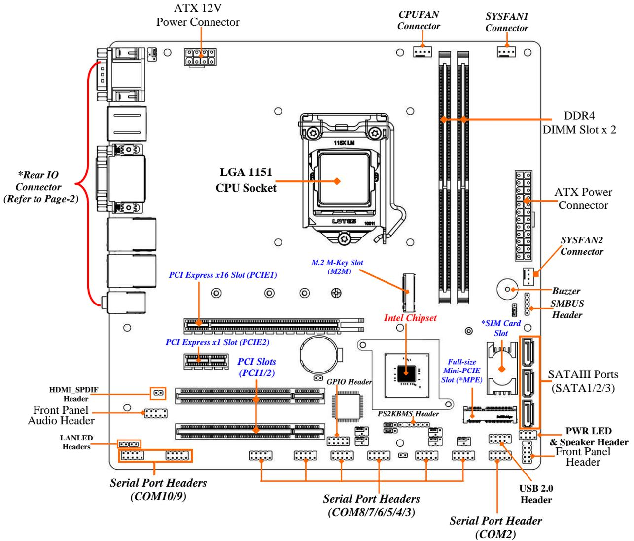
**\*Note:** SIM card slot only work **when** compatible SIM card installed & LAN expansion card installed in MPE Mini-PCIE slot.
