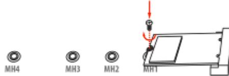
5. Tighten up the screw to secure the module into the M.2 connector. Make sure not overtighten the screw to avoid possible damage to the module.
