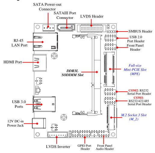
Note: 1. SODIMM module should be 1.35V DDRIII SODIMM and not exceeding 8GB total capacity.
