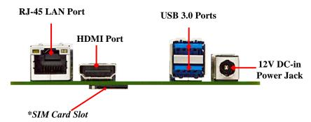
**Note: SIM card slot** is on the back side of the board and only works **when** compatible SIM card installed & 3G LAN card installed in full-size Mini-PCIE (**MPE**) slot.
