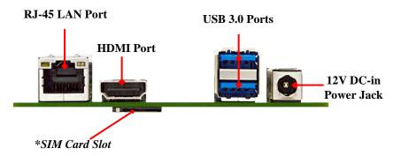
**Note: SIM card slot** is on the back side of the board and only works **when** compatible SIM card installed & 3G LAN card installed in full-size Mini-PCIE (MPE) slot.
