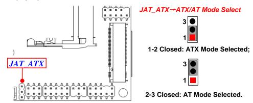
\*ATX Mode Selected: Press power button to power on after power input ready; AT Mode Selected: Directly power on as power input ready.
