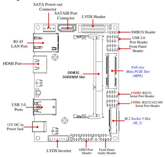
**Note:** 1. SODIMM module should be 1.35V DDRIII SODIMM and not exceeding 8GB total capacity.
