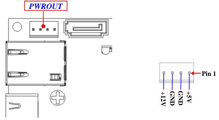
**Warning:** Make sure that Pin-1 of compatible SATA Power connector is inserted into corresponding Pin-1 of **PWROUT** connector to avoid possible damage to the board and hard disk driver!
