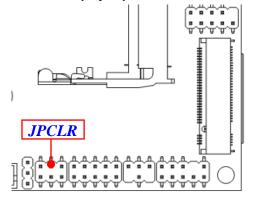
Pin (3&4) of JPCLR→ Reset RTC for Clear Flash
