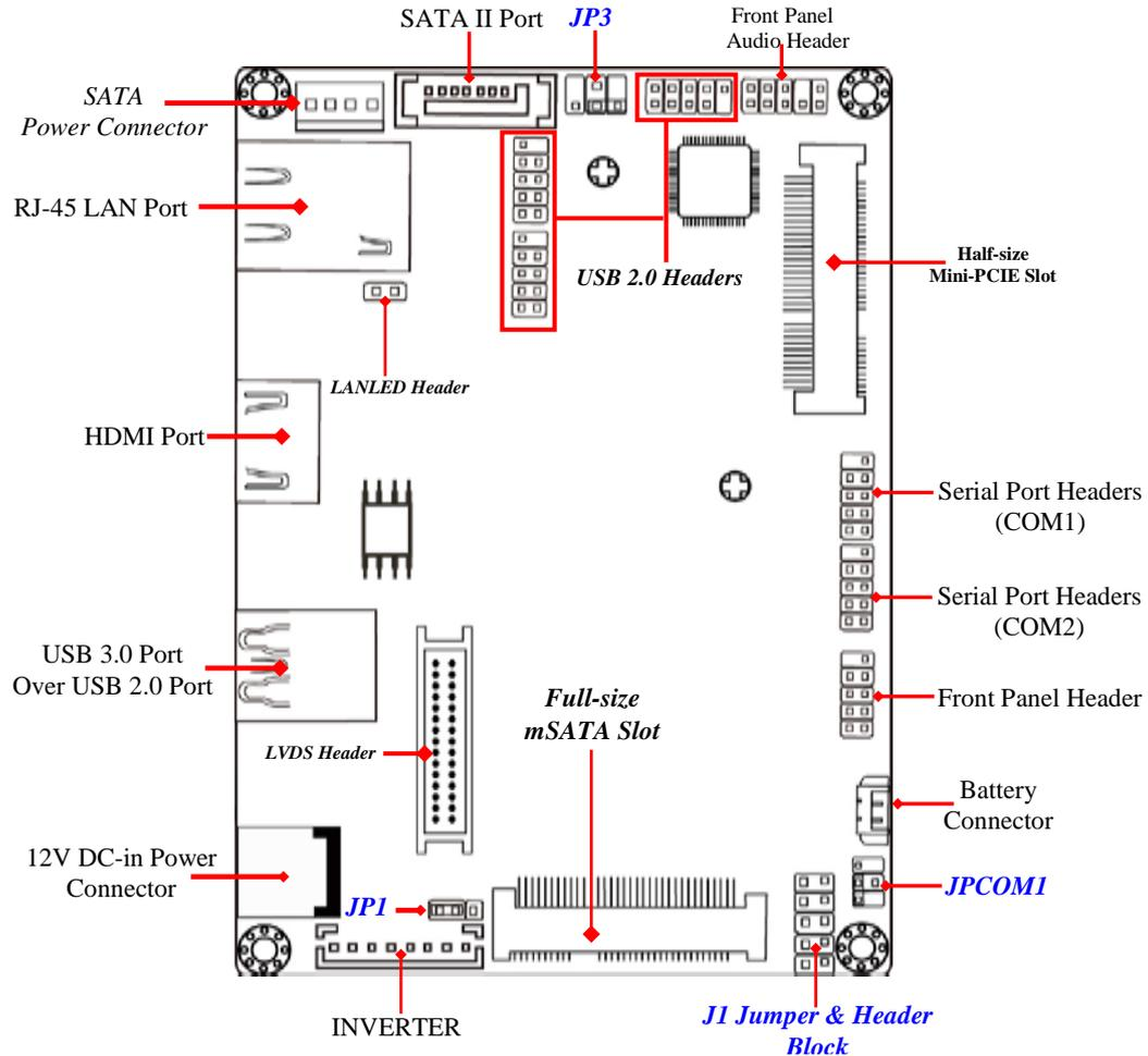
**\* Note:** The 10-Pin J1 block is only optional for the latest upgraded PCB version. The previous J1 block only come with 8 pins.
