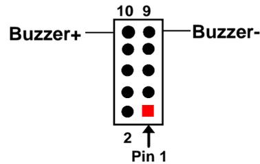
*\* Note: Pin-9 & Pin-10 of J1 block is only optional for the latest upgraded PCB version. The previous J1 block only come with 8 pins.*
