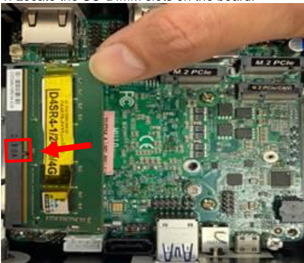
2. Insert the gold-figure side of the compatible SO-DIMM into the slot at a 30 degree angle. See to it that the break of the module fit into the notch of the slot.
