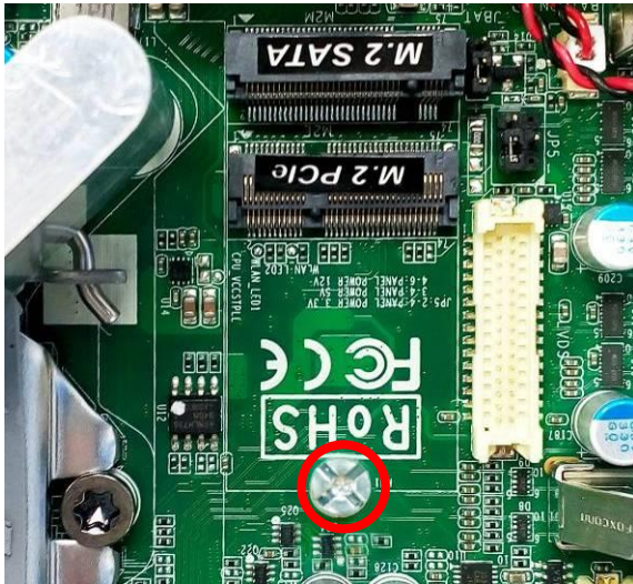
3. The screw post located on the lower side is reserved for M.2 PCIe card.
