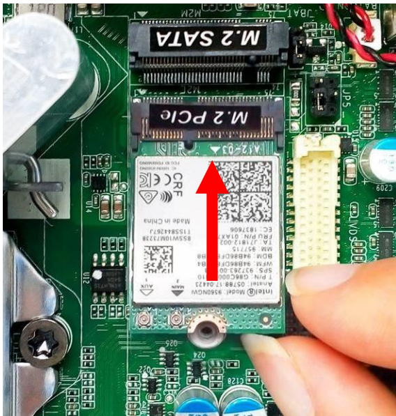
5. Insert the gold-figure side of compatible card into M.2. PCIe slot. See to it that the golden-figure side is fully inserted into the slot.
