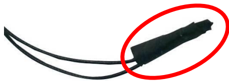
7. The metal hats on the end of the antenna string are sealed by acetate tape to avoid possible damage to the system.
