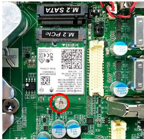
6. Lock the card to the board by tightening up the screw post to the marked spot.
