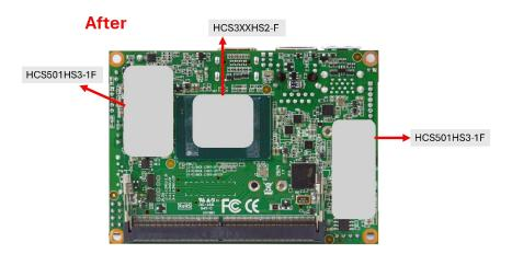
2. Place the motherboard with the side containing the thermal pad facing upward. Align the screw holes on the motherboard with those on the heatsink, then fasten screws properly using a screwdriver.
